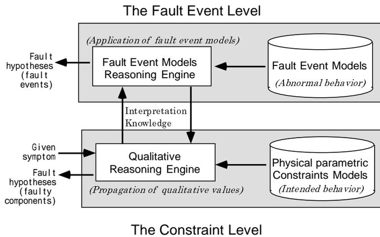
**Figure 3: The framework of the integrated diagnosis method**
