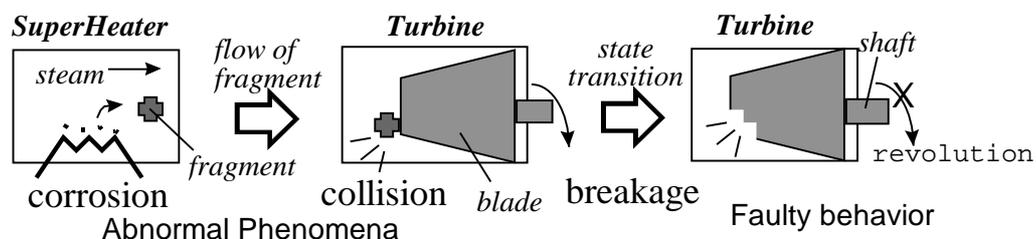
Figure 1: An example of causal chains including non-physical parametric faults
