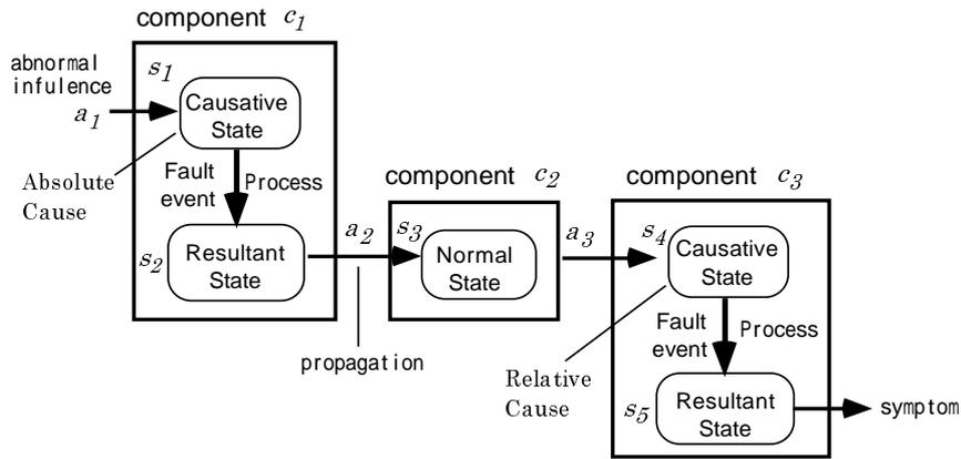
**Figure 2: An example of a causal chain of fault events**
